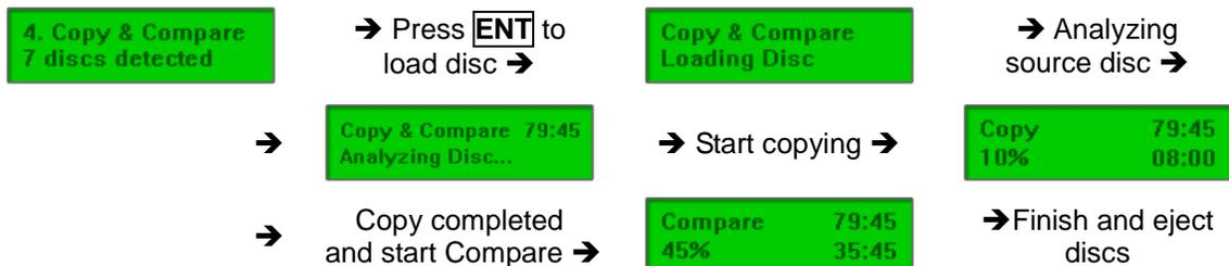
6. Once the compare process is completed, the trays will automatically eject discs that have passed the Copy & Compare process.
