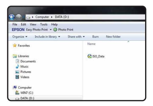
Turn on the "ISO" duplicator machine which has USB connection to built-in HDD. There is a switch located on the back of duplicator. Please turn the USB switch ON, and connect the duplicator to your computer USB port with a USB cable. The computer will see the duplicator's HDD and install it automatically as an external hard disk drive.
